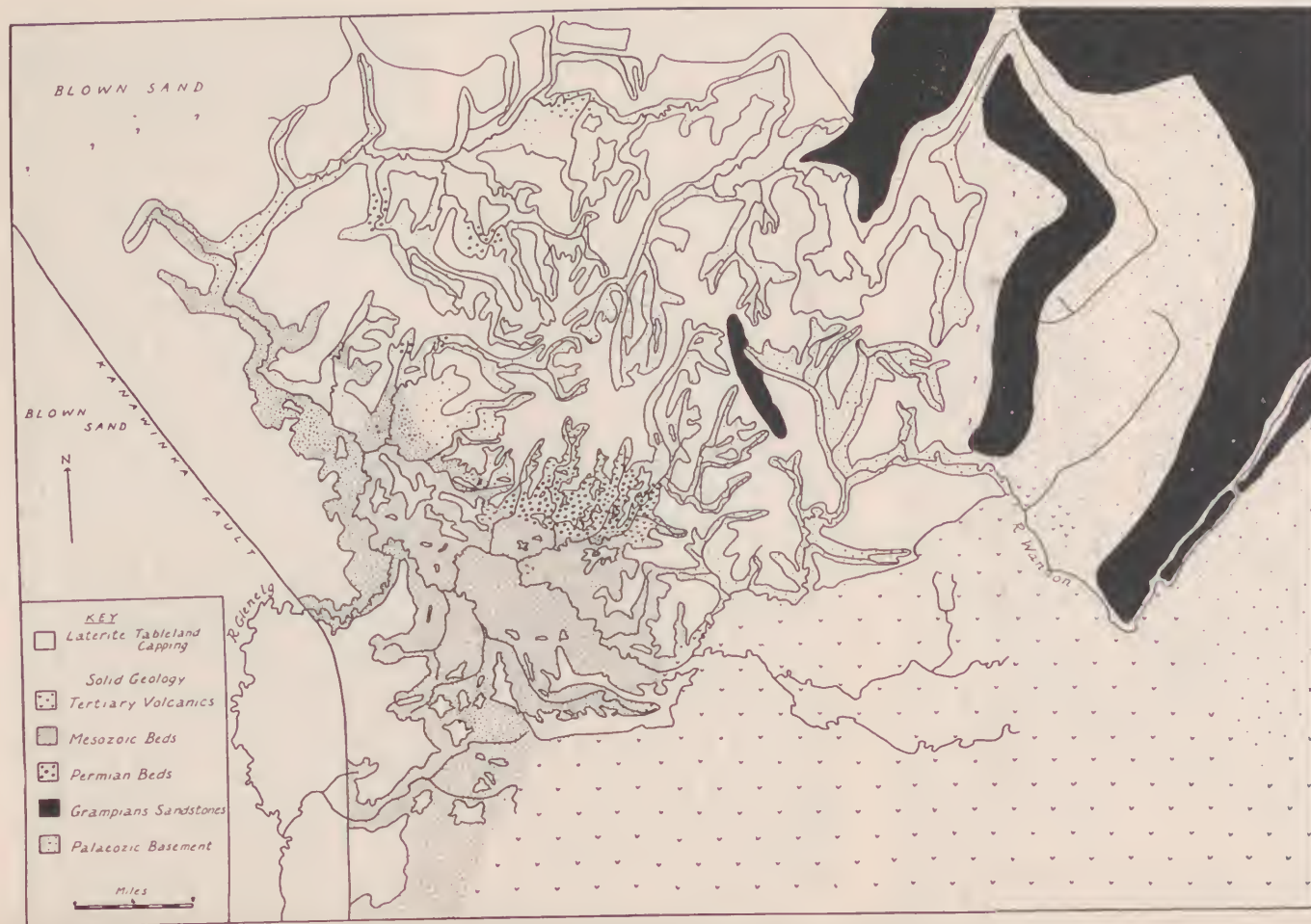
FIG. 2.—The laterite tableland cappings in relation to the geology of the Dundas area.
